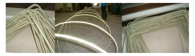
Generally, pairs of U or C or L - shaped bars are more economical. Z - shapes or gull- wing type configurations are not very economical. A 90- degree bend with 12db bar diameter, pigtail used to shorten development length is just as effective as a J- shape as per ACI 440.1R.
