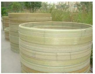
Due to the low modulus of the Pulwell GFRP bar, it is possible to pack the rebars especially small sizes (below 12.7mm) into coils with several hundred meters per roll, or field form the bar into large radius curves.
